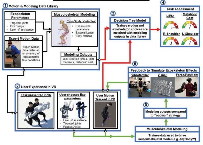
FIGURE 3 Virtual reality-based motor training framework for the use of exoskeletons
