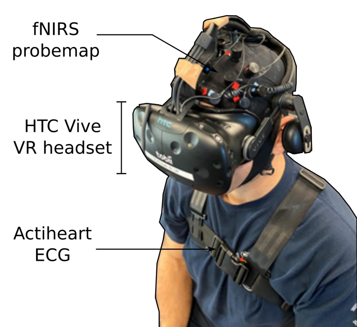
Fig. 2: (a) The experiment workflow during the VR valve sequence execution task. (b) Snapshot of an instrumented participant (RIGHT).
